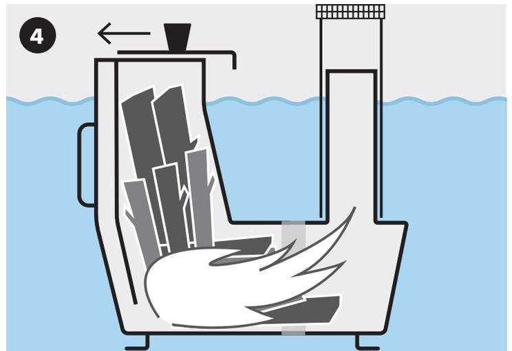
4 When the fire is going, fill the stove with logs, as the picture shows. Add logs every 20 minutes or so. Keep a strong fire in the stove. Close the stove lid completely when the water have reached a pleasant temperature.
