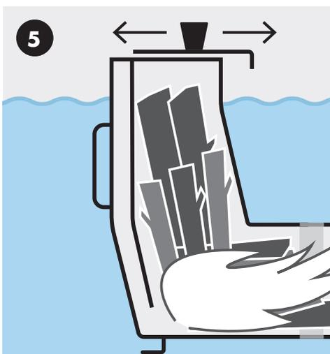
5 If the water gets cold - adjust the hatch to allow for more draught, but no more than the picture shows. You can also put more logs on the fire during a bath.
