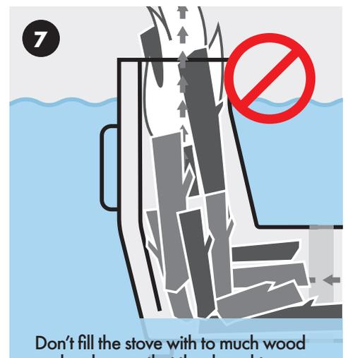
7 Don't fill the stove with too much wood and make sure that the draught doesn't run the wrong way, making the flames escape through the stove opening. And lastly - make sure that the fire and embers have died out completely before emptying the tub.
