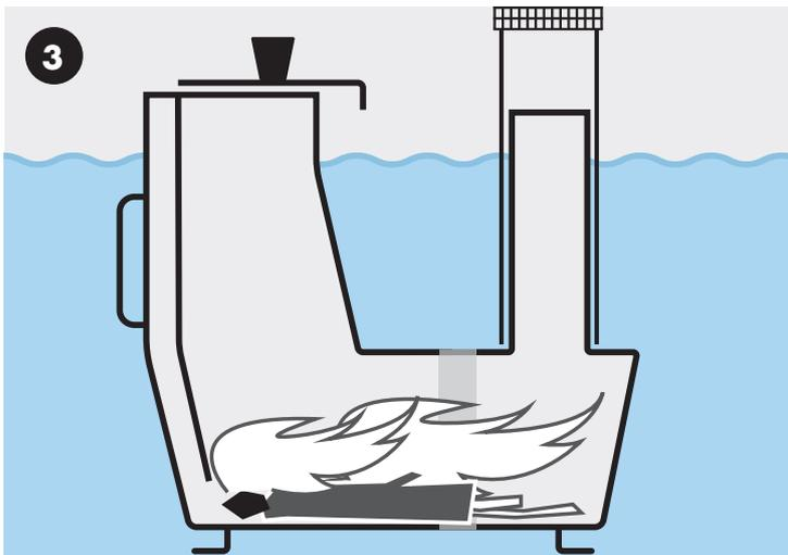
3 Add small logs and tinder sticks horizontally in the stove. Put the big logs to the sides and the smaller tinder in the middle. Add another piece of burning birch bark/firestarter close to the burn plate. The flames should always escape the stove through the chimney pipe, not the stove opening.
