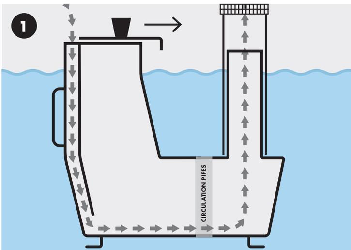
1 This is the way the air should flow through the stove. Use the hatch to adjust the draught. Never open the hatch more than the picture shows, or use the stove without the hatch. Always have water in the tub when using the stove, about as much water as the picture shows.
