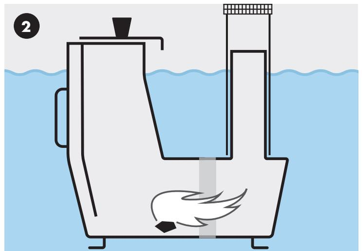
2 Set fire to a piece of birch bark or a firestarter. Do not use lighter fluid. Place the birch bark or firestarter in the stove, as close to the circulation pipes as possible. Let it burn for a minute before adding more tinder.
