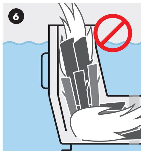
6 Again, never leave the hatch off the stove, since this may result in flames escaping the stove and scorching the wooden frame of the tub, or parts of the interior.
